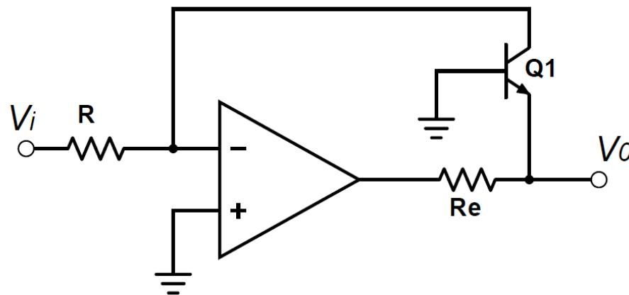
$$\frac{V_o + V_{BE}}{R_E} + g_m \cdot V_{BE} + \frac{V_{BE}}{r_\pi} = 0$$
