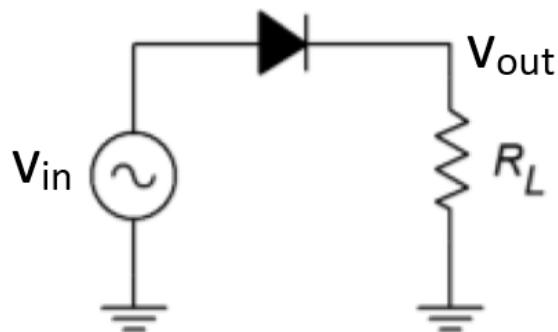
$$v_{out} = \begin{cases} v_{in} - V_\gamma & \text{za } v_{in} > V_\gamma \\ 0 & \text{za } v_{in} \leq V_\gamma \end{cases}$$
