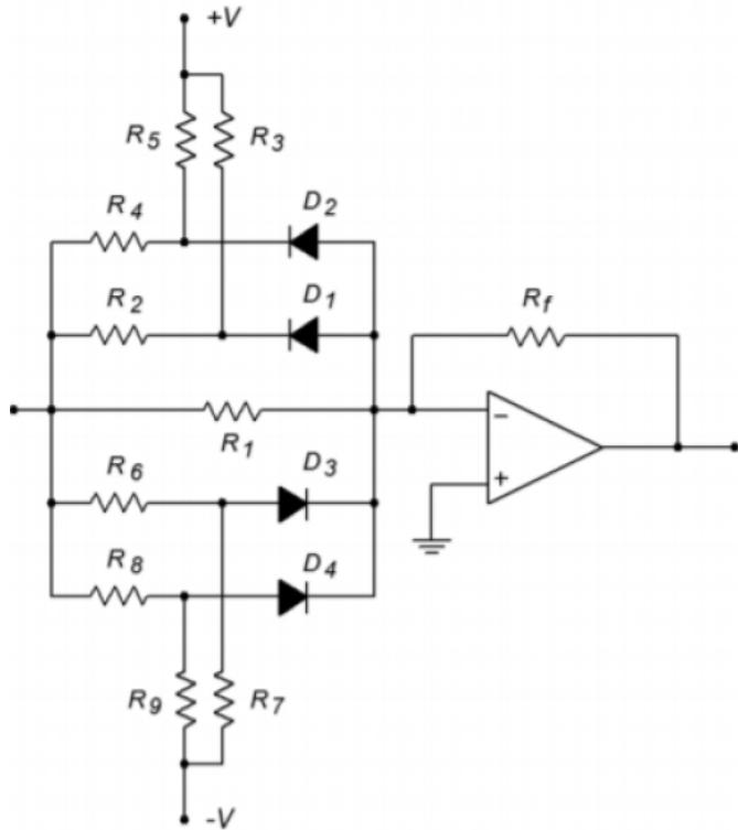
$$v_{out} = -\left(\frac{R_f}{R_1 || R_6}\right) \cdot v_{in}$$
